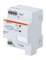
The DG/S 1.64.1.1 DALI-Gateway (1fold) can install up to 64 DALI devices both via 16 flexible DALI (orange lined group) and KNX lighting groups (green dotted lined group), each with one or more DALI participants. Control and Monitoring via KNX. Control and status feedback can also be carried out via Broadcast. 16 independent Lighting scenes are available.
