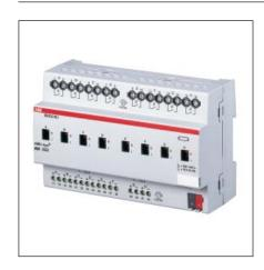
The ABB i-bus® Switch/Dim Actuators with a rated current of 16 A are EIB / KNX modular installation devices in ProM design for installation in the distribution board on 35 mm mounting rails. The connection to the ABB i-bus® is implemented via a bus connection terminal.
